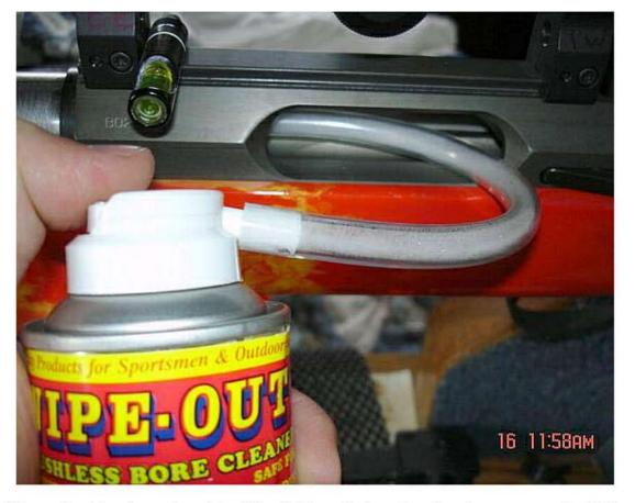
When using this setup and applying Wipe-Out from the breech end, make sure you put a 180° bend in the tube while applying it, that way you won't launch chunks of foam straight out of the muzzle. Give the can a half-second shot and wait for the spaghetti to stop flowing from the muzzle. Pull the tube out of the chamber and let Wipe-Out do the work. Also, after application, rinse the tubing out with water, as Wipe-Out will degrade it after a few days.
